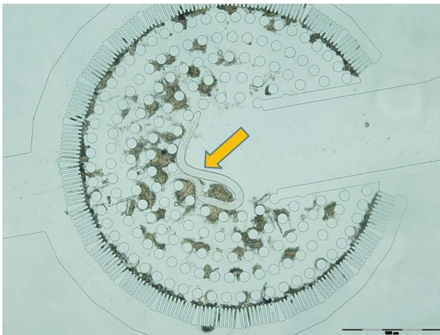
Figure 2. The second filtration area of the microfluidic device. The picture shows the trapped Trichinella spp. larvae (yellow arrow) in the second filtration area between the retained residues (brown color). × 4.
